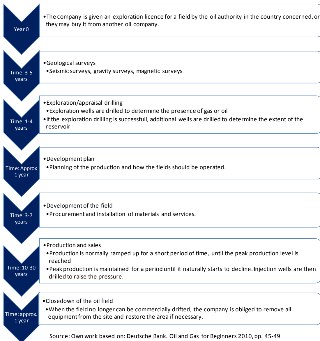
Figure 1.8 Typical life cycle of an oil field
